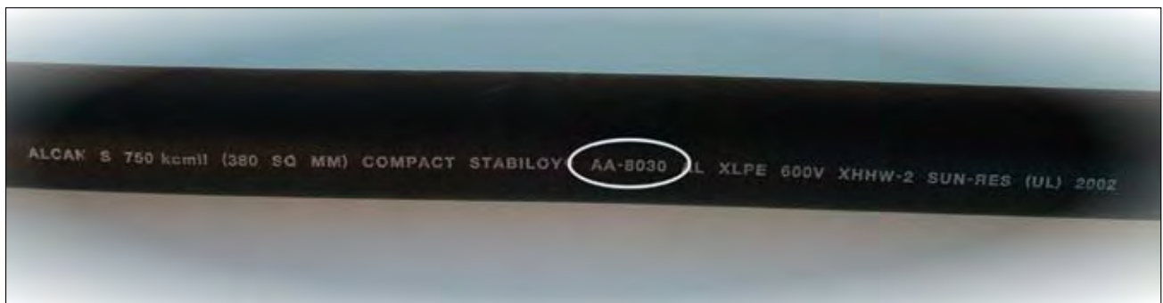
Photo 2. Legend on commercially available AA-8000 conductor
