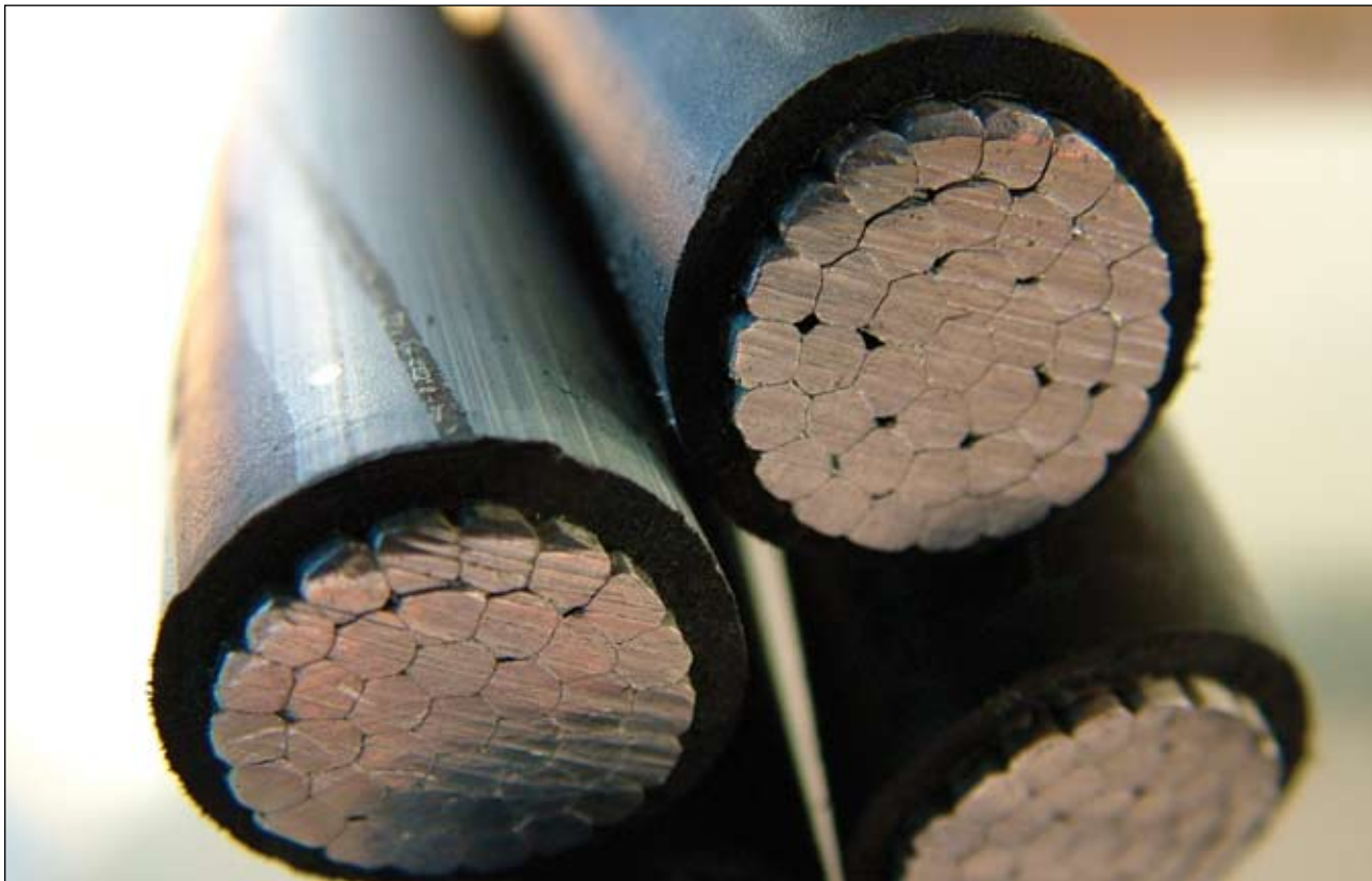
Photo 3. Compact stranded aluminum conductor
