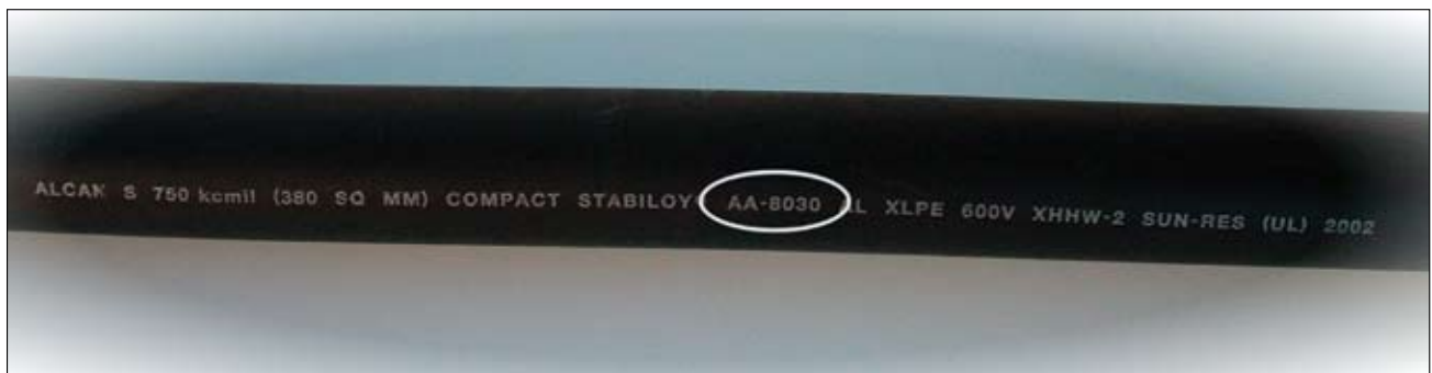
Photo 2. Legend on commercially available AA-8000 conductor
